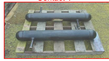
First coating with Rust Contact V Finishing with Aqua Sealer
