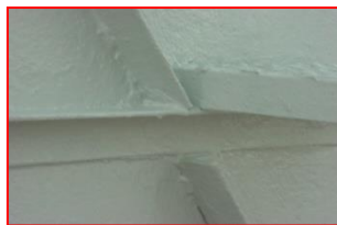
Rusted Surface after application of Rust Contact V
