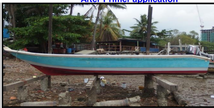
After Hull Coat Application
