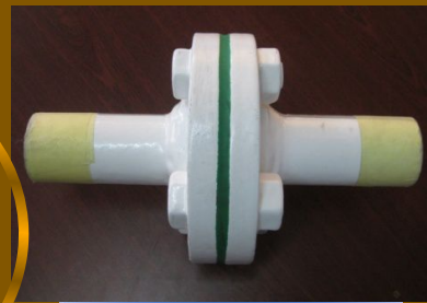
Application of PU in between flanges for corrosion protection
